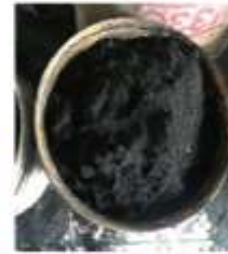
Rubber chips made by crushing waste tires then make it to powder
